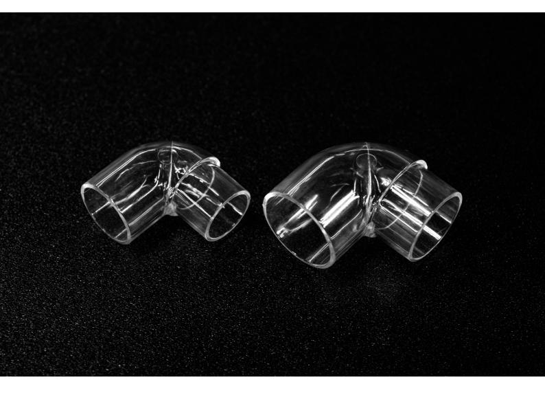
The material of L parts used in NeoFlow and related products was changed from PETG to PC (polycarbonate), which significantly reduced the possibility of breakage. The thickness is the same
